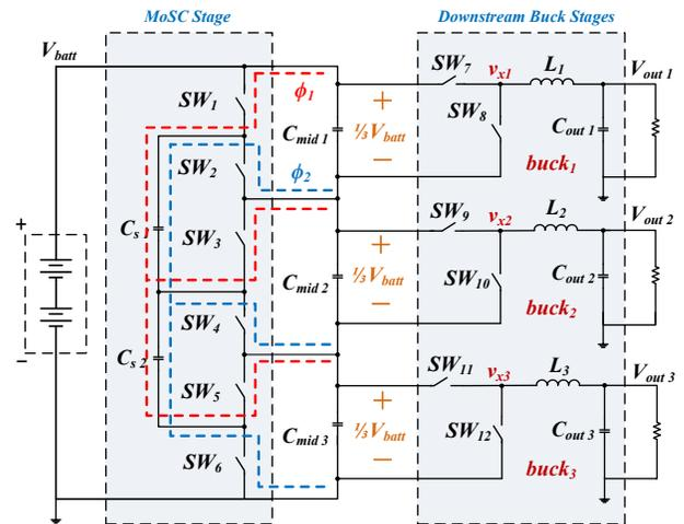
Fig.3 Triple output MoSC-based power management module.
