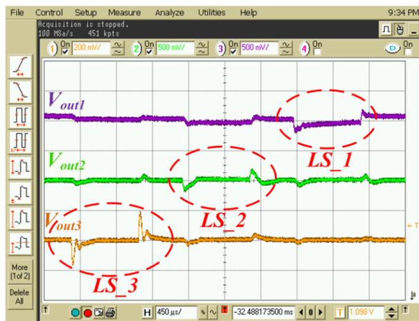
Fig.9 Cross regulation between output voltages. Actual load steps are marked in red dotted circles ( $LS_1$  to  $LS_3$ ). Ch1:  $buck_3$  output voltage,  $V_{out3}$  (200 mV/div); Ch2:  $buck_2$  output voltage,  $V_{out2}$  (500 mV/div); Ch3:  $buck_1$  output voltage,  $V_{out1}$  (500 mV/div).
