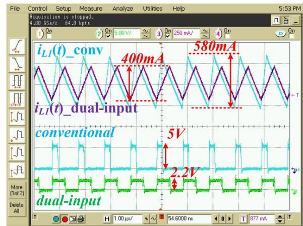
Fig.6 Inductor currents and switching node voltages of the conventional and MoSC-based dual-input downstream stage for 1 V output. Ch2: switching node,  $v_{s3}$  (5 V/div); Ch3: inductor current (250 mA/div).
