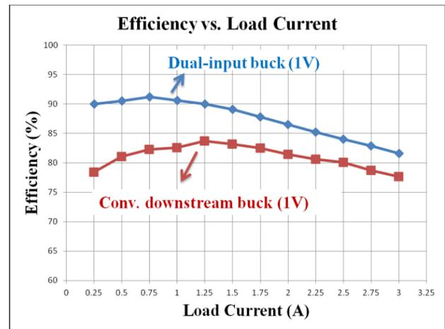
Fig.7 Efficiency comparisons of the MoSC based dual-input buck architecture and the conventional downstream converter.
