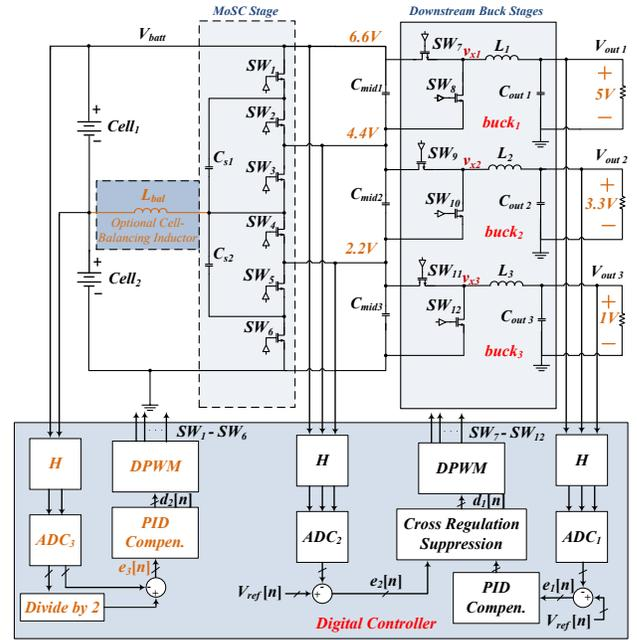
Fig.4 Practical implementation of triple-output MoSC-based power management module and its controller.
