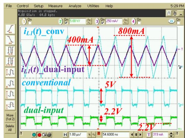
Fig.5 Inductor currents and switching node voltages of the conventional and MoSC-based dual-input downstream stage for 3.3 V output. Ch2: switching node,  $v_{x2}$  (5 V/div); Ch3: inductor current (250 mA/div).
