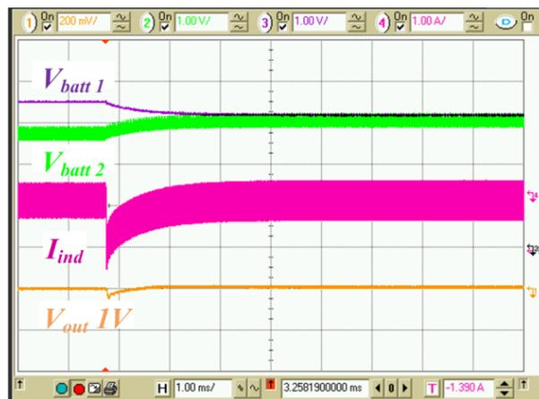
Fig.11 Performing battery cell balancing while regulating the output voltage. Ch1:  $buck_3$  output voltage,  $V_{out3}$  (200 mV/div); Ch2: bottom battery cell voltage (1 V/div); Ch3: top battery cell voltage (1 V/div); Ch4: current of the cell balancing inductor,  $L_{bal}$  (1 A/div).
