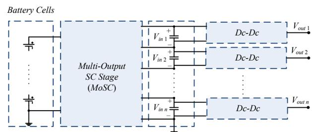
Fig.2 Multi-output SC (MoSC) based power management system.
