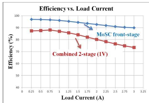
Fig.8 Measured efficiency of MoSC front-stage alone and combined 2-stage, from battery source to 1V output, of the proposed architecture.
