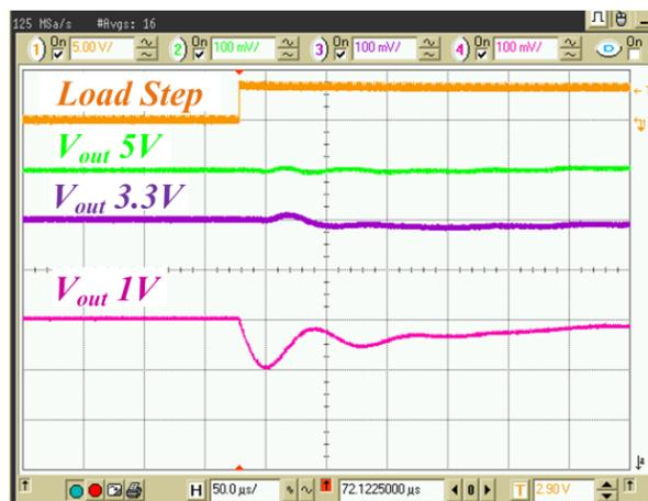
Fig.10 Significant suppression of cross regulation problem. Ch1: load step signal; Ch2:  $buck_1$  output voltage,  $V_{out1}$  (100 mV/div); Ch3:  $buck_2$  output voltage,  $V_{out2}$  (100 mV/div); Ch4:  $buck_3$  output voltage,  $V_{out3}$  (100 mV/div).
